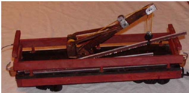
A 40 ft "rail car" by Bud Quinn. Before the days of welded rails, standard rail lengths were 39 ft in order to fit on a 40 ft flat bed car.
