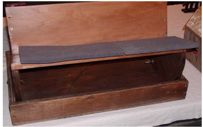
A rotating fixture for holding cars and locomotives while they are being worked on by Bud Quinn.
